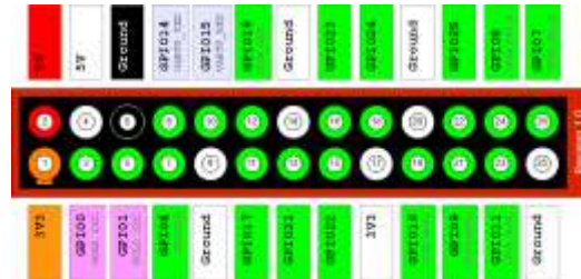
Fig.4: GPIO pin configuration
